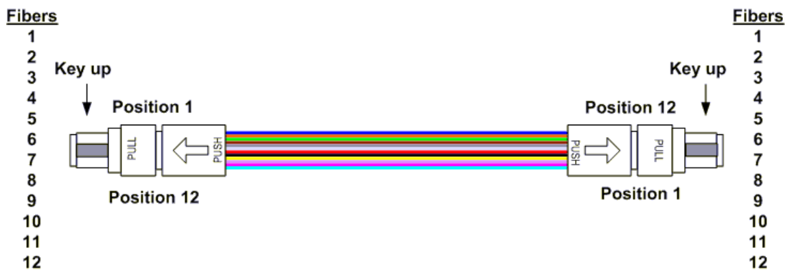
Figure 8 - Type-B array patch cord (key-up to key-up)
