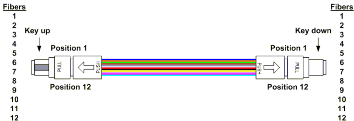
Figure 7 - Type-A array patch cord (key-up to key-down)
